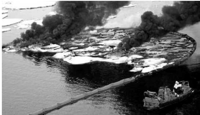
Fig. 1. In situ oil slick burning in presence of ice for test purposes Source: EPR Guide Oil Spill Response in Snow and Ice Conditions in the Arctic.
