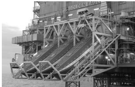
Fig. 3. Offshore aluminium alloy, strengthened hull free fall lifeboats
