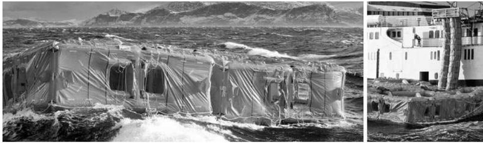
Fig. 2. Marine Evacuation System
