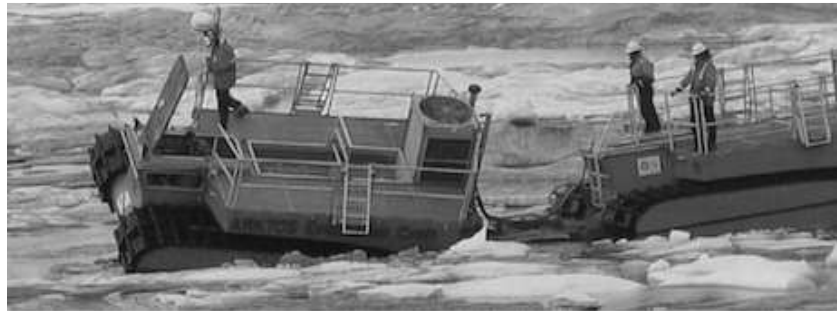
Fig. 10. Arktos moving through broken ice.
